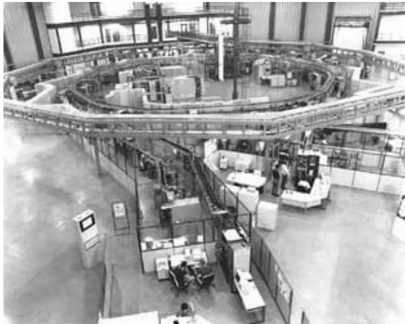
Figure 6: Photograph of the LNLS storage ring, showing the the SAXS beamline in the forefront. The storage ring itself is the central circular structure seen in the top half of the photograph, inside the zigzag wall of concrete blocks used as a protective shield. The outer ring, running above the floor, carries electric power and cooling water for the beamlines.
