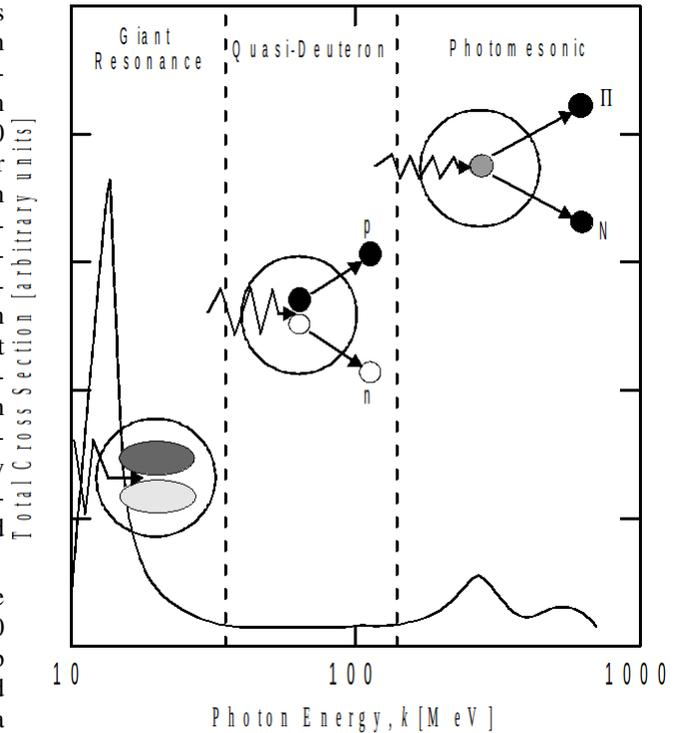
FIG. 1: Showing the primary nuclear photo-interaction according to the incident photon energy. n, neutron; p, proton; N, neutron or proton;  $\Pi$ , mesons  $\pi^0$ ,  $\pi^-$  or  $\pi^+$ ,  $\pi^0\pi^0$ ,  $\pi^-\pi^+$ ,  $\pi^0\pi^-$  or  $\pi^0\pi^+$ .
